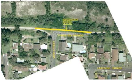
This section was obviously left because of the difficulty of putting the cycleway on the side of an embankment between Tuggerah Parade and the lake foreshore. This section needs to be completed off road to ensure the whole length between Long Jetty and The Entrance is off road.
